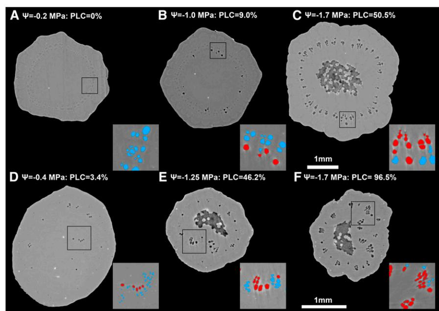
**Figure 1.** Transverse HRCT images of intact *V. vinifera* 'Cabernet Sauvignon' plants at different water potentials: stems (A–C) and petioles (D–F). Insets represent 0.25-mm<sup>2</sup> areas. Functional (gray) and air-filled (black) xylem vessels are represented in blue and red in the insets, respectively. The theoretical loss of hydraulic conductivity for each image is indicated as PLC (%). Bars = 1 mm.
