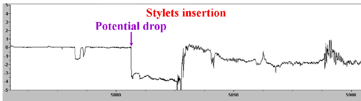
Figure 2. Electrical penetration graph of S. titanus on grapevine showing a potential drop. Abscissa is in seconds, ordinate is in mV.
